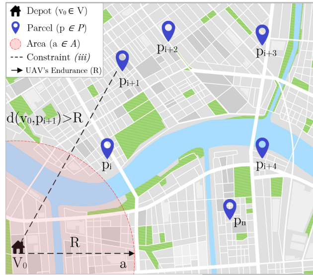
Figure 4.1: A mUCVLMPP instance where a set of parcels p \in P and a depot location v_0 \in V are distributed around a \mathbb{R}^2 Euclidean space. R denotes the UAV's endurance as the farthest distance the UAV can travel considering a return flight to the take off point. The distance constraint is satisfied with d(v_0, p_i) > R .
